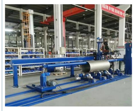
The side beam series equipment is mainly used to complete the circular seam or straight seam welding of the cylindrical workpiece. It has the
