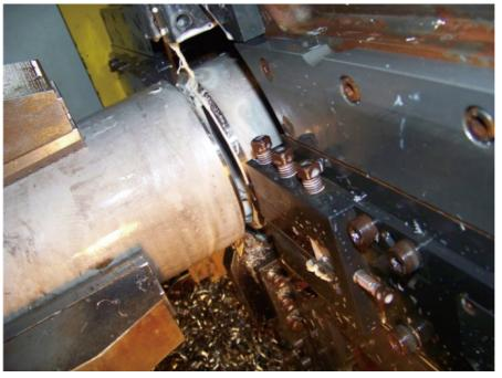
A high-quality and highly efficient integrated cutting and beveling process for small and medium-diameter thin-walled (≤25.4mm) pipes. This process is equivalent in efficiency to 10 sets of band saws and lathes combined. It takes only 2 to 3 minutes for cutting and beveling (two bevels) a 159 × 20 carbon steel pipe. One worker can replace ten workers. The savings in space occupation, labor cost, and electricity cost will recover the investment.
