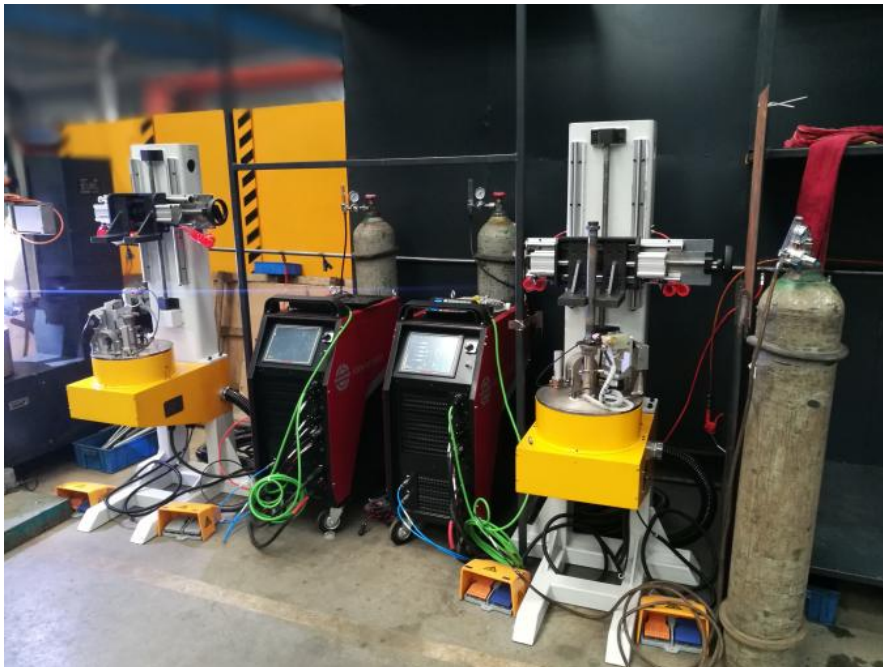
Construction Machinery Industry Hydraulic pipe TIG welding system
