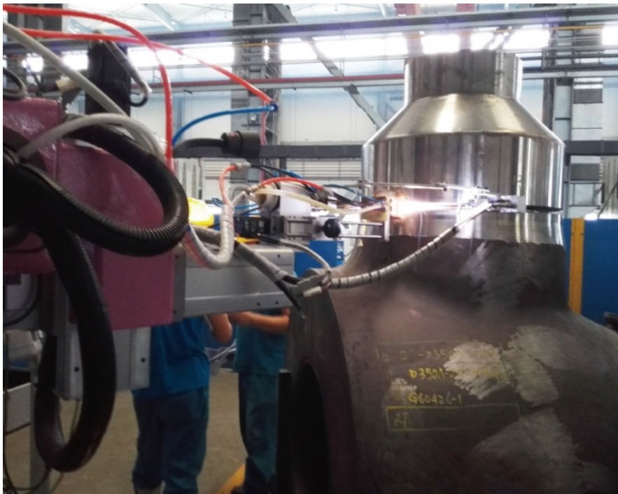
Steam Turbine Industry TIG Narrow Groove Welding System For Valve Casing Connection Application
