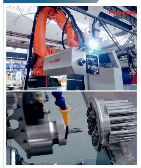
The Huaheng Robot Intelligent Tube Expansion & End-Facing Equipment is equipped with a camera vision and measurement system, enabling the visualization of tube expansion and end-facing processes.
