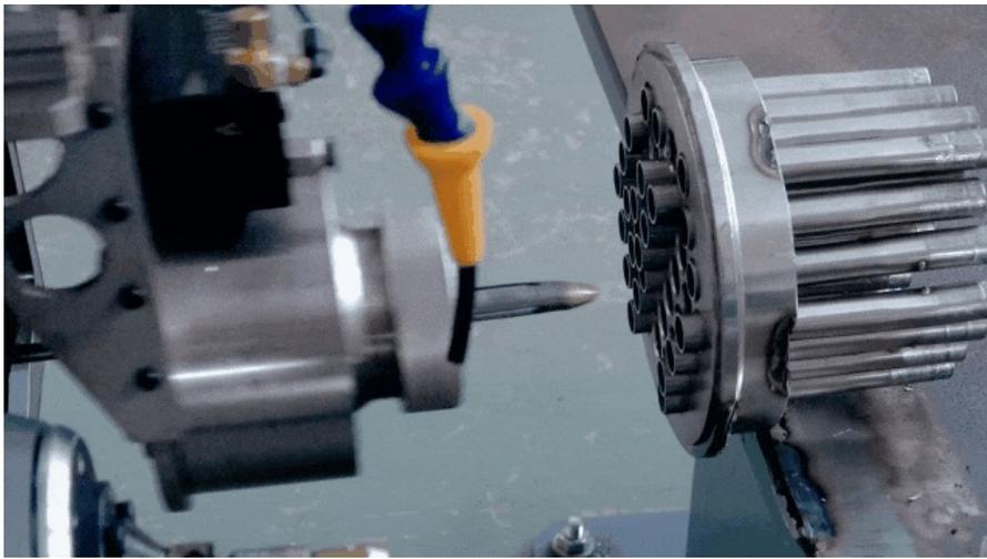
The Huaheng Robot Intelligent Tube Expansion & End-Facing Equipment is equipped with a camera vision and measurement system, enabling the visualization of tube expansion and end-facing processes.
